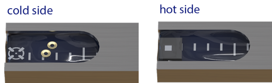
FIGURE 3-57 Transverse Standard (TS) probe Left: cold side; Right: hot side
