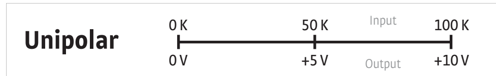
FIGURE 5-4 Output with polarity parameter set to unipolar
