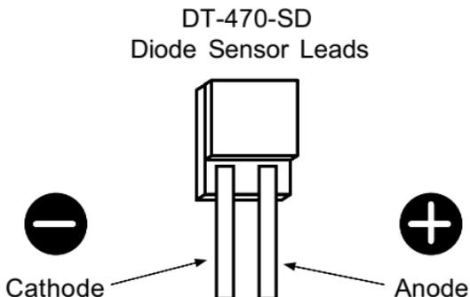
On the DT-470-SD, the base is the largest flat surface. It is sapphire with gold metalization over a nickel buffer layer. The base is electrically isolated from the sensing element and leads; make all thermal contact to the sensor through the base. A thin braze joint around the sides of the SD package electrically connect to the sensing element. Avoid contact to the sides with any electrically conductive material.
