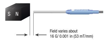
**NOTE:** One of the greatest sources of repeatability errors is variable distance to the probe's active area.
