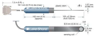
**NOTE:**  $+\Phi$  is designated as that flux passing through the coil, into the side with the Lake Shore logo on the probe handle
