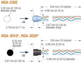
\*The active area is symmetrical with the center line of the assembly and is located approximately 0.030 in behind the front surface of the assembly
