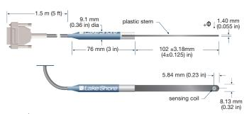
**NOTE:**  $+\Phi$  is designated as that flux passing through the coil, into the side with the Lake Shore logo on the probe handle
