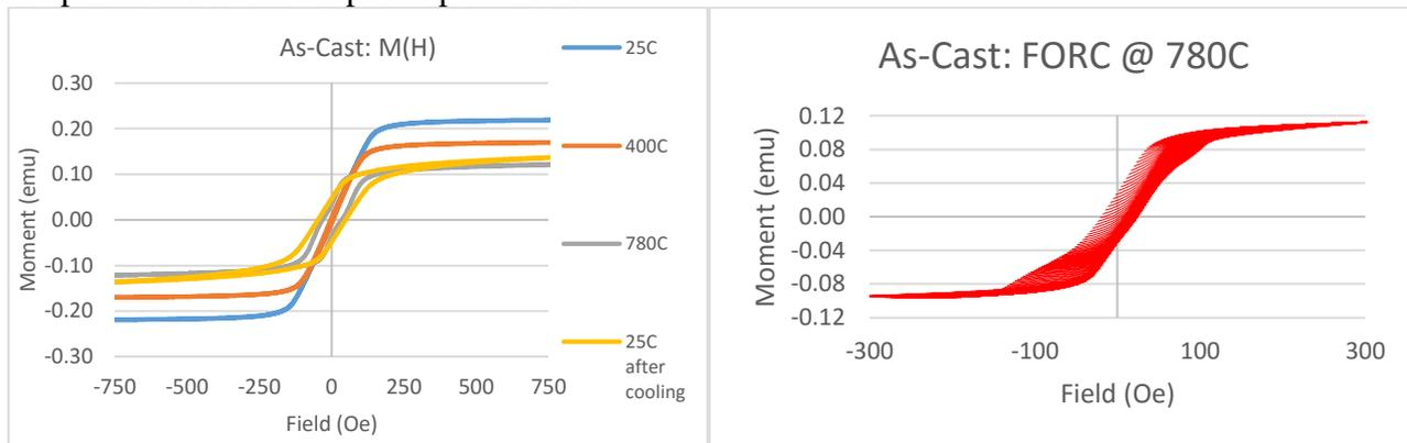
**Figure 5.**  $M(H)$  (left) at 25, 400, 780 and  $25^\circ\text{C}$  after cooling, and the measured FORCs (right) at  $780^\circ\text{C}$  for as-cast FeCo-based nanocrystalline amorphous/nanocomposite sample.
