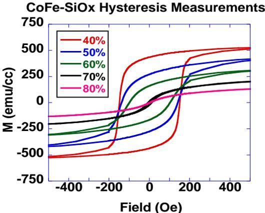
**Figure 1.** Room temperature hysteresis loops for CoFe nanoparticles dispersed in SiO<sub>2</sub> with volume fractions ranging from 40% to 80% (data are volume normalized and presented in emu/cc).
