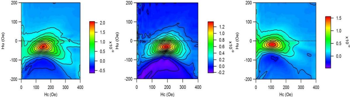
**Figure 2.** Room temperature 2D FORC diagrams for CoFe nanoparticles dispersed in SiO<sub>2</sub> volume fractions of 40% (left), 50% (middle) and 60% (right).
