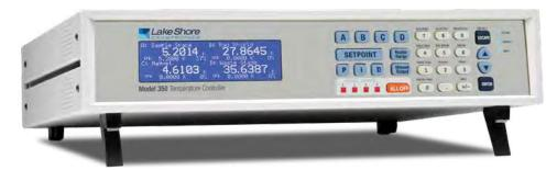
The patented noise reduction input circuitry of the Model 350 is just one reason why this controller works so well for ultra-low temperature (ULT) applications, all the way down to 100 mK. When combined with precision Cernox sensors, this performance-optimized design allows as little as 10 nA of excitation current to be used, minimizing self-heating effects, and ensures best possible measurement accuracy throughout the entire temperature range.
