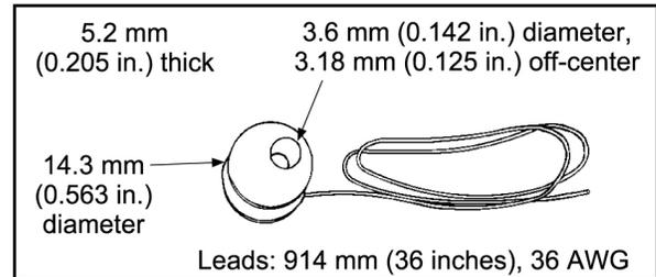
**NOTE:** This package is designed for use up to 325 K (52 °C), subjecting sensor to temperature in excess of this will cause a shift in the sensor values.
