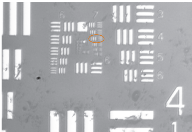
Left: smallest feature visualized (approximately 3 \mu\text{m} ) obtained with a Zoom 70 and coaxial light on a CPX-VF probe station
