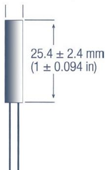
Lake Shore cartridge heaters can be used with all of our temperature controllers. Heaters have wattage ratings in dead air. In cryogenic applications, these cartridge heaters can handle many times the rated value if properly heat sunk or in liquid.
