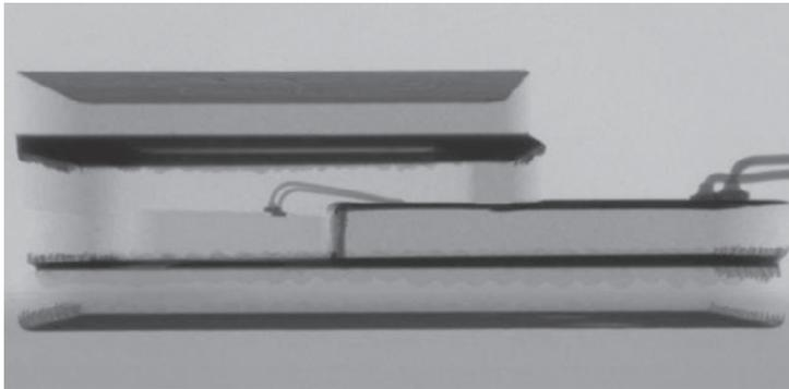
Lake Shore x-rays each sensor to verify the quality of the die attachment and to ensure sufficient clearance between the internal wires and lid.
