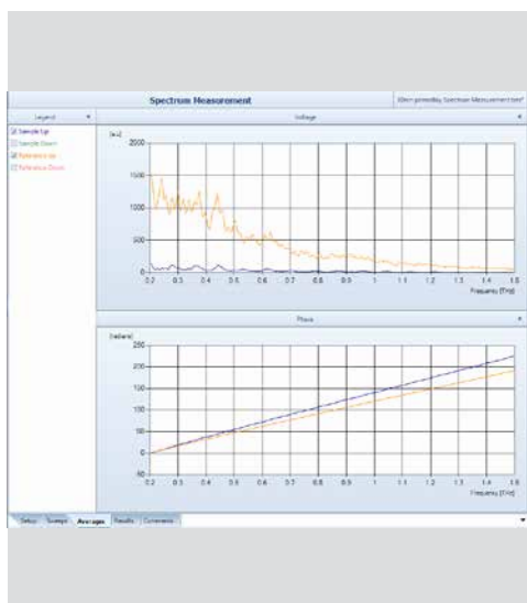
⑦ Sample, reference, and background data are automatically acquired for each profile point
