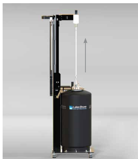
⑨ Remove insert from cryostat and exchange sample
