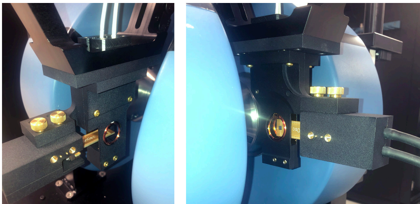
CPW sample holder for NanOsc spectrometer integration
